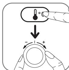
Press **°C** key. Set the desired temperature by turning the selector for the desired temperature from 80°C to 240°C.
