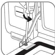
Open the door. Make sure that it is placed on a stable surface: turn your oven by 90°.
