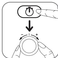
Press **START** key. Set the duration of cooking by turning the selector until the desired time. The digital display tells you the time in hours and minutes (e.g.: 0: 5).
