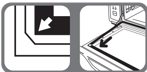
Replace the inner pane (check that the markings are on the inner surface of the door). Take care to position the glass correctly: the **rounded corners should be on** the lower side (near the door hinges). Fit the upper corners into the notches (see arrows). Replace the mounting flanges. Screw it back loosely.
