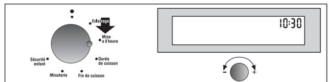
2- When the minutes flash, set the central button by turning to the "-" or "+" symbol. Confirm by pressing the central button.
